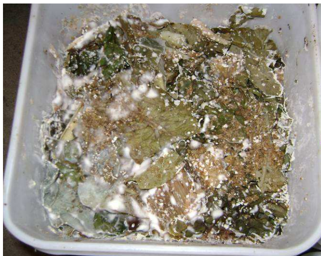
Figure 2 - Photograph of trial Ferm 1 post-fermentation, showing white threads associated with fungal or bacterial (Actinomycetes) growth
